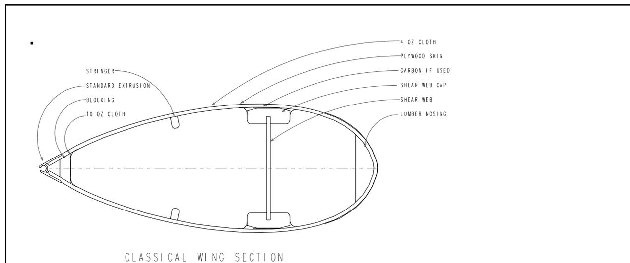
The stitch and glue mast must by definition have thin walls and usually a defining longitudinal spar or shear web that the walls are bent around. A wing mast with that longitudinal spar does have the disadvantage of creating extremely high aspect ratio panels. These panels are liable to fail sooner than lower aspect ratio ones. A stitch and glue mast is however built with the fewest number of pieces, which can speed construction time.
