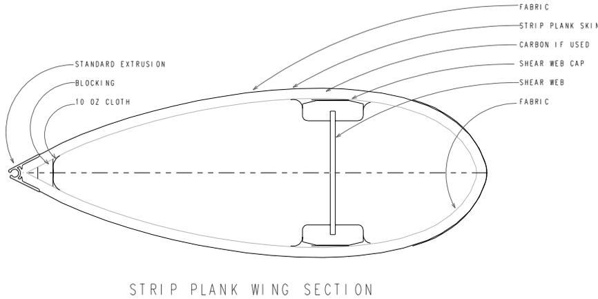
The strip plank wing masts have ideal foil sections and can be of any size as the material is not forced to bend around any shape such as a shear web. Excessive time to build and higher weight are the main objections to strip masts. These do have a large number of pieces to be joined together and additional fiber reinforcement is needed. Unfortunately that reinforcement must be oriented across the primary load direction and does not directly help resist those loads .
